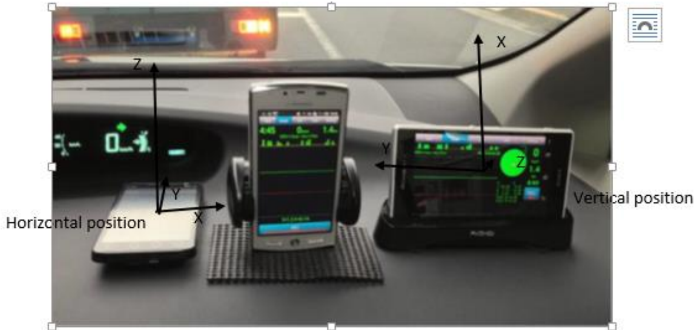
Fig 9: Road bump measurement using smartphone
